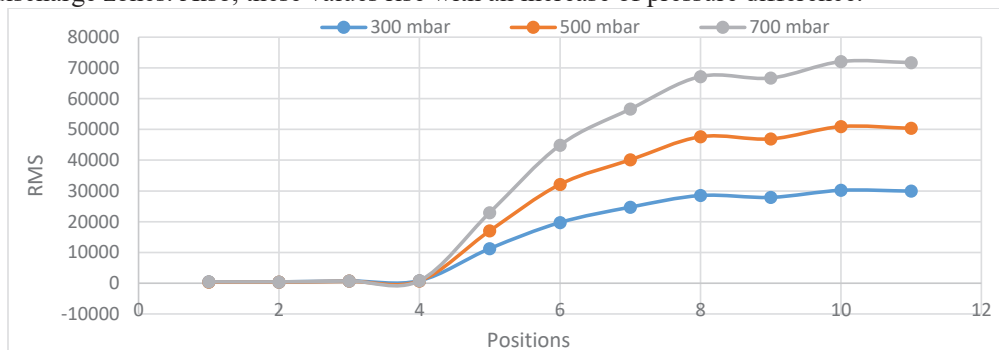
Figure 16: Root Mean Square (RMS) of effective pressure zones at 1800 rev/min and different pressure difference.
